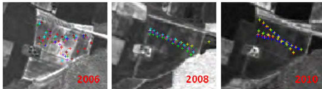
Figure 2.6- Illustration of the dynamics of the itinerary for collecting ground data over the Auradé site, in 2006, 2008 and 2010. For these years, winter wheat was cultivated. The 'crosses' represent the registered GPS points where measurements were performed. Each different color represents a date of measurement over the vegetative cycle.
