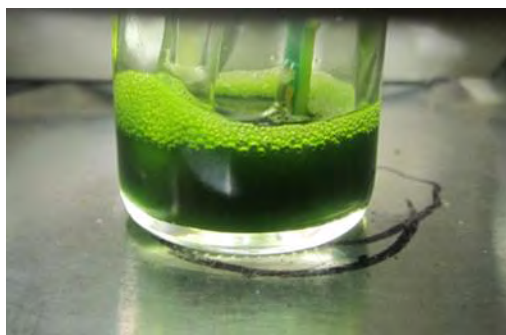
Figure 5.2. Silicon-based oxygen sensor in algal solution.
