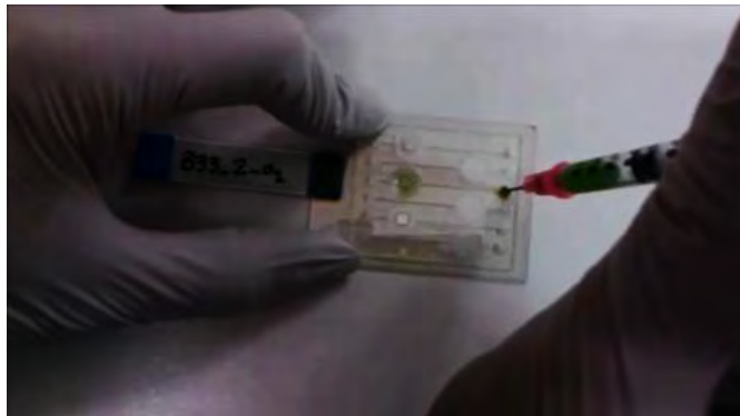
Figure 4.19. Test solution injection in lab-on-chip device.
