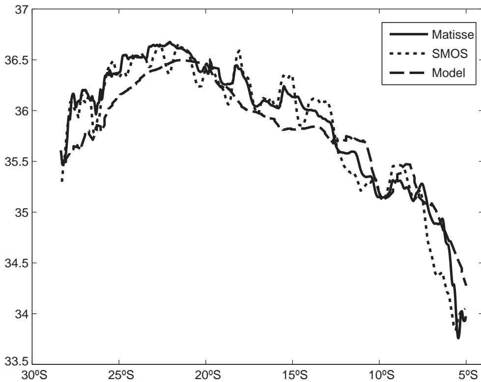
Figure 2 Comparison between near-surface salinity data derived from (black line) the TSG instrument installed on board M/V Matisse and the collocated SSS: (dashed line) modelled and (dotted line) SMOS values. The Matisse salinity values were obtained during 20-27 February 2011 along the northern shipping line shown in Figure 1a.
