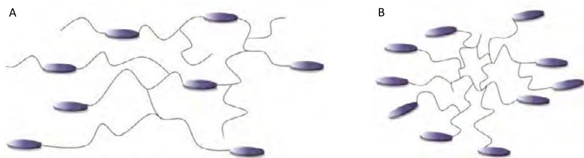
Figure I.14. Schematic representation of the two general classes of liquid crystal hyperbranched polymers; main-chain (A) and side-chain (B).
