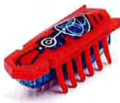
Figure 5.9: A self-propelled robot of the brand Hexbug: a small battery-powered electric engine triggers the vibration of the device. The bended plastic legs offer differential friction with the substrate. As a result, the device moves ahead. Due to unbalanced bending, most of these devices move along circles of various radii.
