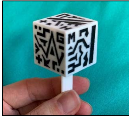
Figure 3. 3D-printed augmented reality cubic marker used in the augmented reality system.
