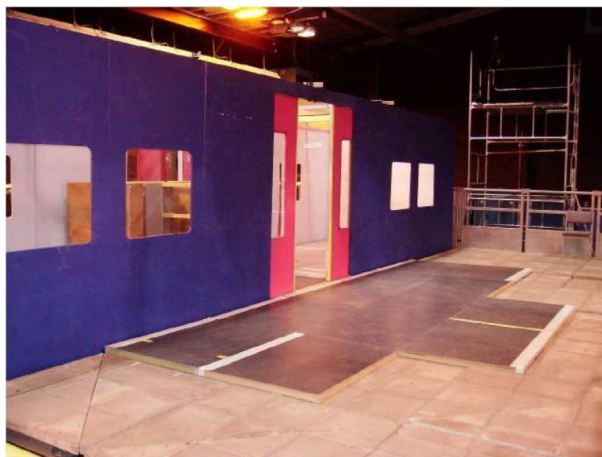
Figure 1. Pedestrian Accessibility Movement Environment Laboratory (PAMELA) configured as a London Underground carriage to study effect of door width and vertical gap [12].
