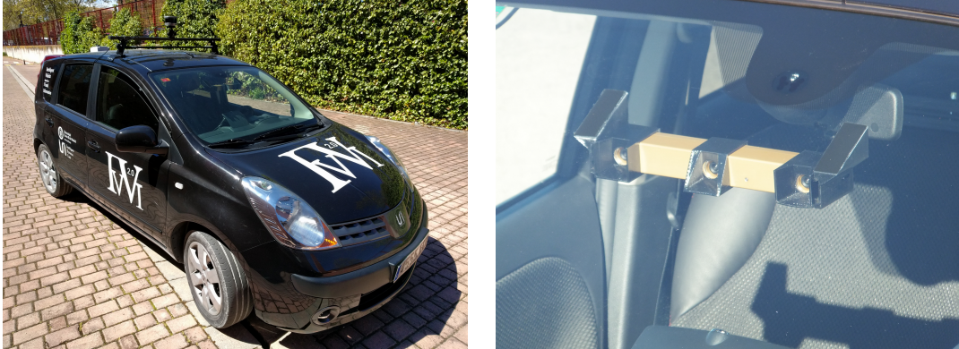
Figure 1: IVVI 2.0, Intelligent Vehicle based on Visual Information: (a) external view; (b) detail of the trinocular stereo vision system mounted on the windshield.
