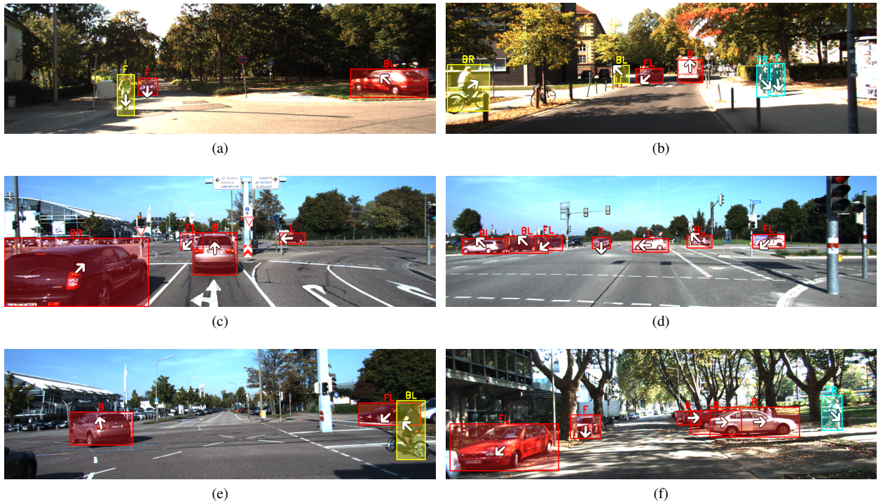
Fig. 9. Examples of detections with viewpoint estimation on the KITTI test dataset. Class is encoded using color: Car , Cyclist and Pedestrian classes are represented as red, yellow, and blue, respectively. The pseudo-continuous viewpoint estimation is depicted as an oriented white arrow at the center of the obstacle, while the predicted bin is provided above each bounding box as a combination of front (F), back (B), left (L) and right (R).
