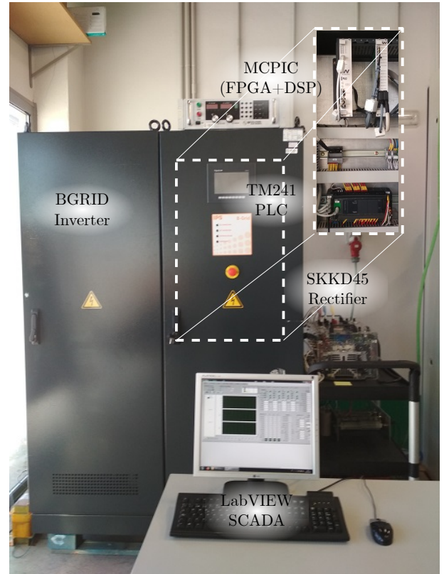
Fig. 13. Overview of the set-up used in the real-time experiments.
