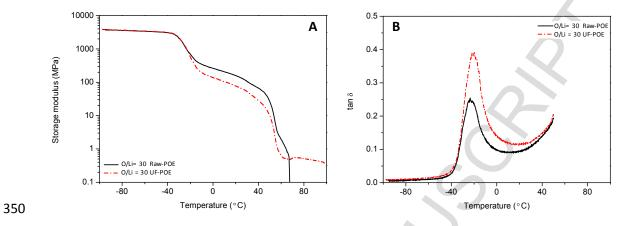
Figure 1. Storage modulus E' (A) and Tan  $\delta$  (B) vs temperature at 1Hz for raw and
