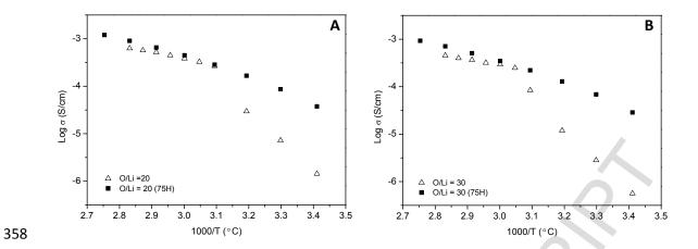
**Figure 3**. Comparison of conductivity performance of ultrafiltrated and partial hydrogenated polymer electrolytes with a O/Li ratio of 20 (A) and 30 (B).
