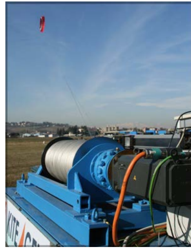
FIGURE 1.7: KiteGen KSU1. Rated Power 40KW [56].
