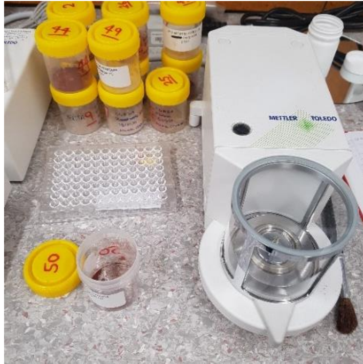
Figure 10. Weighing of freeze dried blood samples into tin capsules, using a Mettler Toledo XP6 microbalance.
