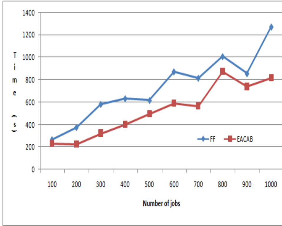
Figure 4.13: Simulation with Enersim 1 : Makespan with EACAB compared to dynamic first fit (FF)
