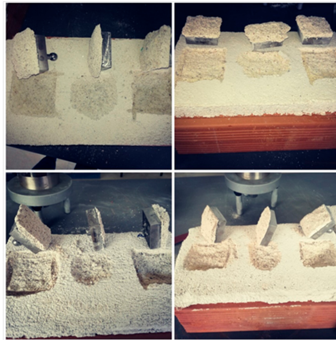
Figure 9. Images of cohesive fractures observed in the studied mortar coatings after performing the pull-off test.
