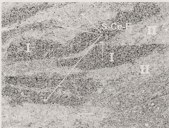
FIG. 11.—Backscattered electron image of clay deposits bearing APS minerals. Svanbergite-Ce-florencite (S-Ce-F). (I) High-porosity zones with alunite, halloysite, diaspore, and svanbergite-Ce-florencite. (II) Low-porosity zones rich in pyrophyllite, kaolinite, micas, svanbergite-Ce-florencite, and heavy metals. Middle Lithofacies, Las Aguilas Formation, Cuchilla de Las Aguilas, Barker area.
