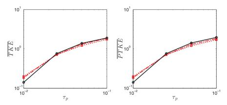
**Fig. 14.** Turbulence with radiation and gravity: Lagrangian with 64 particles per cell (black full) versus Eulerian (red) simulations with  $64^3$  (dotted line) and  $128^3$  (dot-dashed line) cells. Mean Total Kinetic Energy (left) and Particle Total Kinetic Energy (right) versus  $\tau_p$ . (For interpretation of the references to color in this figure legend, the reader is referred to the web version of this article).
