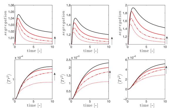
**Fig. 8.** Decaying turbulence with radiation and no gravity: Lagrangianwith 64 particles per cell (black full) versus Eulerian (red) simulations. Segregation (top) and temperature variance (bottom) versus time for  $\tau_p = 0.01$ , 0.05 and 0.1. The arrows indicate increasing mesh size from 64<sup>3</sup> to 256<sup>3</sup>. (For interpretation of the references to color in this figure legend, the reader is referred to the web version of this article).
