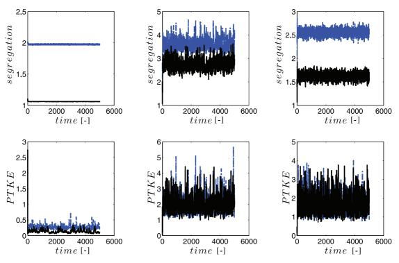
**Fig. A.16.** Turbulence with radiation and gravity: effect of the number of particles on the statistics of the Lagrangian simulations. Segregation (top) and Particle Total Kinetic Energy (bottom) versus time for  $\tau_p = 0.01$ , 0.1 and 0.8, for 1 particle per cell (dot-dashed line) and 256 particles per cell (full line).
