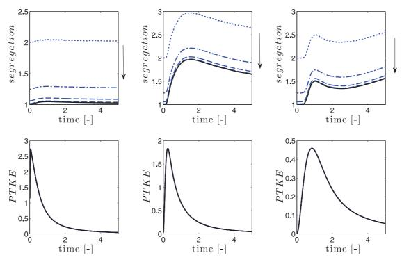
**Fig. 2.** Decaying turbulence without radiation: effect of the number of particles on the statistics of the Lagrangian simulations. Segregation (top) and Particle Total Kinetic Energy (bottom) versus time for  $\tau_p = 0.01$ , 0.1 and 0.8. The arrows indicate increasing number of particles by a factor of 4 from 1 particle per cell to 256 particles (black full line) per cell. For the PTKE, all the results are overlapping.
