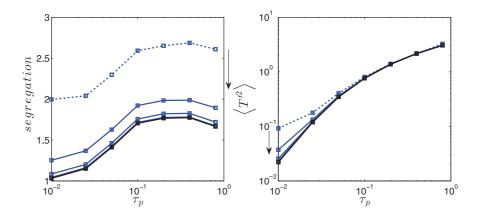
**Fig. 7.** Decaying turbulence with radiation and no gravity: effect of the number of particles on the statistics of the Lagrangian simulations. Maximum segregation (left) and Temperature variance (right) versus  $\tau_p$ . The arrows indicate increasing number of particles by a factor of 4 from 1 particle per cell to 256 particles (black full line) per cell.
