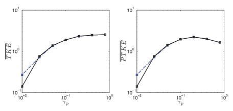
**Fig. 11.** Turbulence with radiation and gravity: effect of the number of particles on the statistics of the Lagrangian simulations. Mean Total Kinetic Energy (left) and Particle Total Kinetic Energy (right) versus  $\tau_p$ , for 1 particle per cell (dot-dashed line) and 256 particles per cell (full line).
