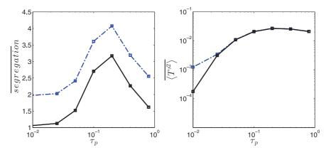
**Fig. 10.** Turbulence with radiation and gravity: effect of the number of particles on the statistics of the Lagrangian simulations. Mean segregation (left) and temperature variance (right) versus  $\tau_p$ , for 1 particle per cell (dot-dashed line) and 256 particles per cell (full line).
