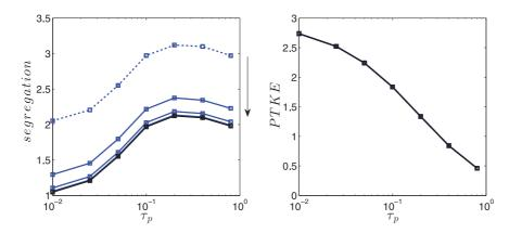
**Fig. 3.** Decaying turbulence without radiation: effect of the number of particles on the statistics of the Lagrangian simulations. Maximum segregation (left) and Particle Total Kinetic Energy (right) versus  $\tau_p$ . The arrow indicates increasing number of particles by a factor of 4 from 1 particle per cell to 256 particles (black full line) per cell. For the PTKE, all the results are overlapping.
