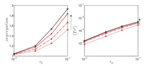
**Fig. 9.** Decaying turbulence with radiation and no gravity: Lagrangian with 64 particles per cell (black full) versus Eulerian (red) simulations. Maximum segregation (left) and temperature variance (right) versus  $\tau_p$ . The arrows indicate increasing mesh size from 64<sup>3</sup> to 256<sup>3</sup>. (For interpretation of the references to color in this figure legend, the reader is referred to the web version of this article).
