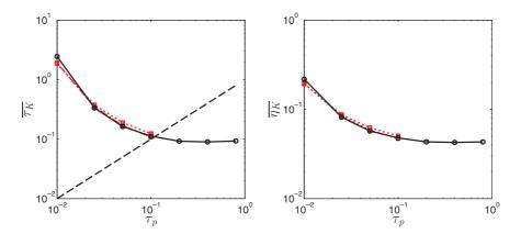
**Fig. 15.** Turbulence with radiation and gravity: Lagrangian with 64 particles per cell (black full) versus Eulerian (red) simulations with  $64^3$  (dotted line) and  $128^3$  (dot-dashed line) cells. Kolmogorov time (left) and length (right) scales versus  $\tau_p$ . The dashed line corresponds to a Stokes number based on the Kolmogorov time scale equal to one. (For interpretation of the references to color in this figure legend, the reader is referred to the web version of this article).
