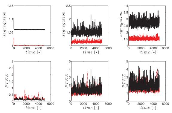
**Fig. A.18.** Turbulence with radiation and gravity: Lagrangian with 64 particles per cell (black full) versus Eulerian (red) simulation with 64 cells. Segregation (top) and Particle Total Kinetic Energy (bottom) versus time for  $\tau_p = 0.01$ , 0.05 and 0.1.
