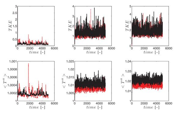
**Fig. A.19.** Turbulence with radiation and gravity: Lagrangianwith 64 particles per cell (black full) versus Eulerian (red) simulation with 64 cells. Total Kinetic Energy (top) and temperature variance (bottom) versus time for  $\tau_p = 0.01$ , 0.05 and 0.1.
