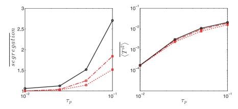
**Fig. 13.** Turbulence with radiation and gravity: Lagrangian with 64 particles per cell (black full) versus Eulerian (red) simulations with  $64^3$  (dotted line) and  $128^3$  (dot-dashed line) cells. Mean segregation (left) and temperature variance (right) versus  $\tau_p$ . (For interpretation of the references to color in this figure legend, the reader is referred to the web version of this article).
