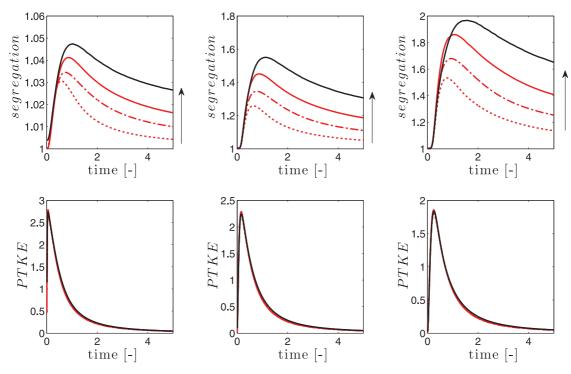
**Fig. 4.** Decaying turbulence without radiation: Lagrangian with 64 particles per cell (black full) versus Eulerian (red) simulations. Segregation (top) and Particle Total Kinetic Energy (bottom) versus time for  $\tau_p = 0.01$ , 0.05 and 0.1. The arrows indicate increasing mesh size from 64<sup>3</sup> to 256<sup>3</sup>. (For interpretation of the references to color in this figure legend, the reader is referred to the web version of this article).
