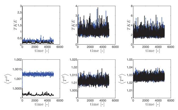
**Fig. A.17.** Turbulence with radiation and gravity: effect of the number of particles on the statistics of the Lagrangian simulations. Total Kinetic Energy (top) and Temperature Variance (bottom) versus time for  $\tau_p = 0.01$ , 0.1 and 0.8, for 1 particle per cell (dot-dashed line) and 256 particles per cell (full line).
