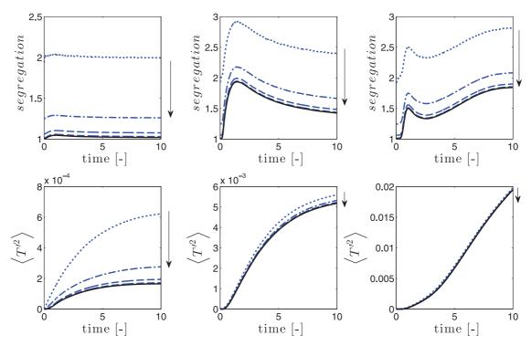
**Fig. 6.** Decaying turbulence with radiation and no gravity: effect of the number of particles on the statistics of the Lagrangian simulations. Segregation (top) and Temperature variance (bottom) versus time for  $\tau_p = 0.01$ , 0.1 and 0.8. The arrows indicate increasing number of particles by a factor of 4 from 1 particle per cell to 256 particles (black full line) per cell.
