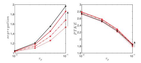
**Fig. 5.** Decaying turbulence without radiation: Lagrangian with 64 particles per cell (black full) versus Eulerian (red) simulations. Maximum segregation (left) and Particle Total Kinetic Energy (right) versus  $\tau_p$ . The arrows indicate increasing mesh size from 64<sup>3</sup> to 256<sup>3</sup>. (For interpretation of the references to color in this figure legend, the reader is referred to the web version of this article).
