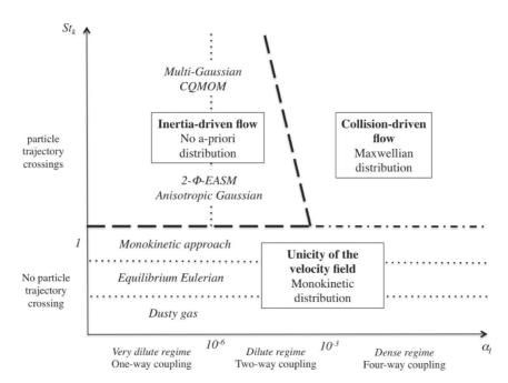
Fig. 1. Existence of an a-priori distribution for particle velocity in turbulent flows: for Stokes number below one the particle velocity distribution is Monokinetic. For Stokes number over one and large volume fraction, the velocity distribution is a Gaussian distribution, following the kinetic theory. For Stokes number over one and very dilute to dilute regime, the velocity distribution cannot be anticipated.
