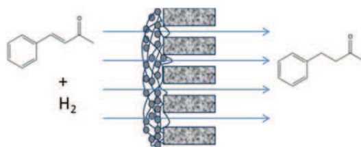
Figure 5: Schematic representation of hydrogenation reaction under catalytic membrane flow-through configuration using a poly(ionic liquid) gel grafted layer load with catalytic palladium nanoparticles.
