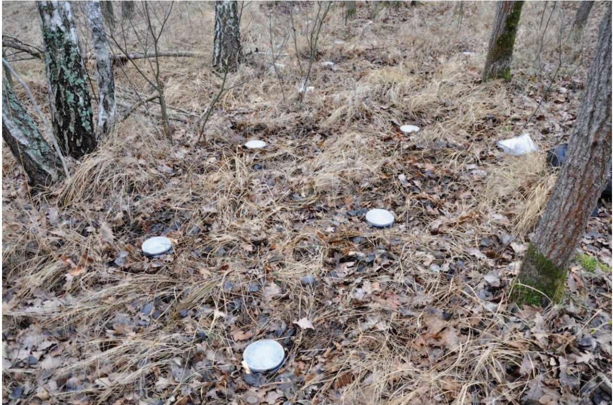
Fig. A.1. The bottom of each microcosm was left open and two 5 x 15 cm windows covered with 1cm nylon mesh were opened on the side at the level of the soil surface, allowing free passage to soil and litter layer invertebrates but avoiding lateral loss of leaf litter. The top of the microcosm was covered with a smaller mesh (0.05 cm), to avoid contamination with autochthonous litter dropping from the canopy. Microcosms were slightly inserted into the top soil, between 0.5 and 1 cm with a distance of about 2 m between individual microcosms. The natural litter removed for microcosm placement was then evenly distributed around the microcosms to provide a continuous litter layer (photos: Jean-Marc Bonzom/IRSN)
