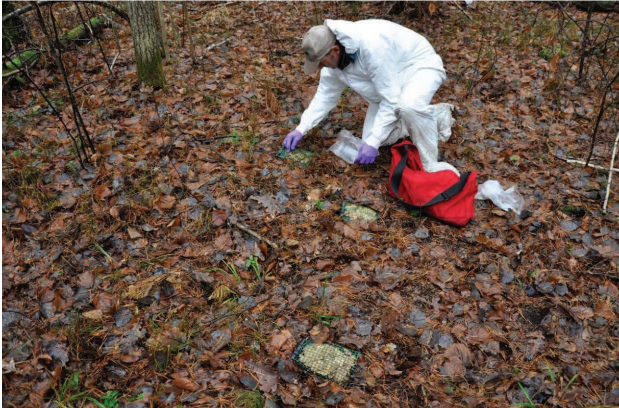
Fig. A.2. The litter bags ( 15 \times 15 cm) at site T were constructed from rigid plastic mesh of 1 cm mesh width. They were placed flat on soil surface with a distance of about 2 m between individual litter bags after the natural litter was removed (photos: Jean-Marc Bonzom/IRSN)
