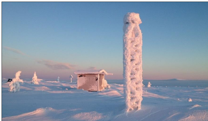
Figure 12. FinnRef station at OLOS in western Lapland as an example how hard rime and snow accumulate on the antenna mast and antenna. (Photo S. Marila)
