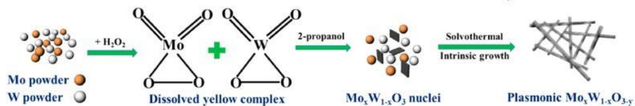
Figure 13. Scheme of synthesis strategy for \text{Mo}_x\text{W}_{1-x}\text{O}_3 by Yin et al. 98 Reprinted with permission from Yin, H.; Kuwahara, Y.; Mori, K.; Cheng, H.; Wen, M.; Huo, Y.; Yamashita, H. Localized Surface Plasmon Resonances in Plasmonic Molybdenum Tungsten Oxide Hybrid for Visible-Light-Enhanced Catalytic Reaction . J. Phys. Chem. C 2017 , 121 (42), 23531–23540. Copyright 2017 American Chemical Society
