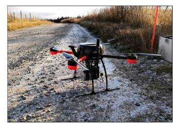
**Figure 5.** (Low-quality version for peer review) GeoDrone X4L multicopter and YellowScan Surveyor LiDAR sensor.
