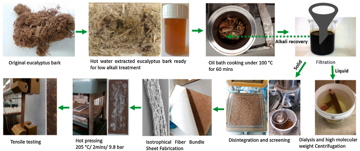
Fig. 1. Experimental flow of fiber bundle separation from eucalyptus bark under mild alkaline conditions and preparation of fiber bundle composites.
