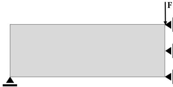
Figure 4.9: Representation of the “MBB” beam with a symmetry boundary condition. Adapted from [Sigmund 2001].
