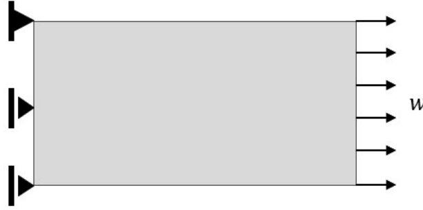
Figure 4.1: Representation of a thin rectangular plane subjected to a superficial load. Adapted from [Kattan 2008].
