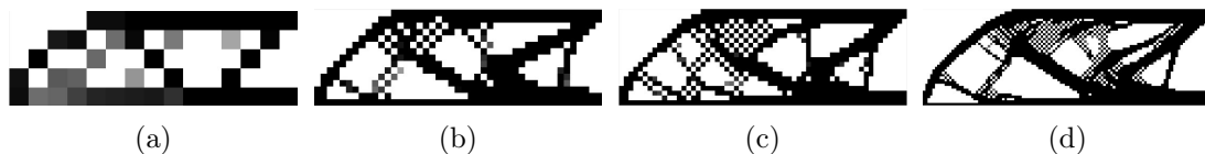
Figure 4.10: Topologies obtained for different meshes without any filtering scheme.
