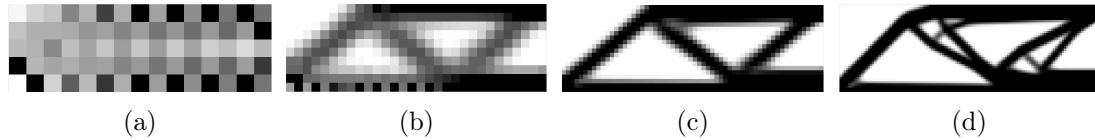
Figure 4.11: Topologies obtained for different meshes using a filtering scheme.
