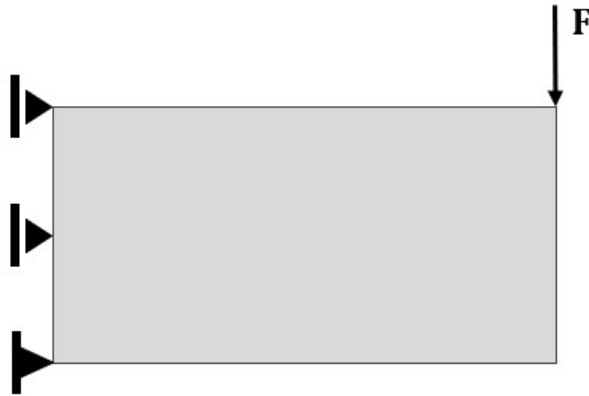
Figure 4.4: Representation of a thin rectangular plate under bending.
