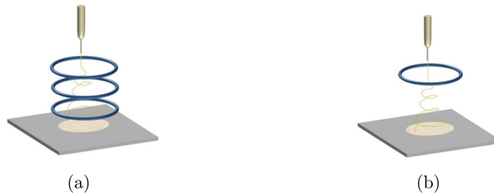
Figure 3.17: (a) Controlled deposition using multiple focusing rings [75]. (b) Controlled deposition using only one focusing ring [77].
