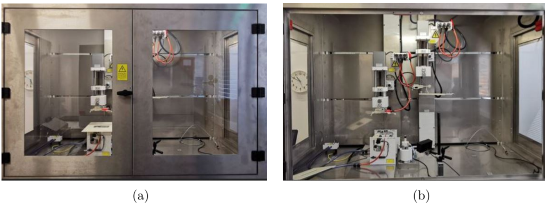
Figure 4.5: Electrospinning Equipment installed in Centre for Mechanical Technology and Automation - TEMA - with door closed (a) and with door opened (b).
