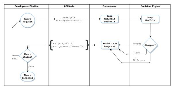
Figure 5.10: API - method to abort an existing security analysis pipeline
