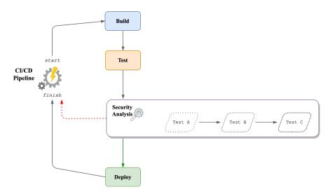
Figure 5.2: Security analysis pipeline in a CI/CD application pipeline
