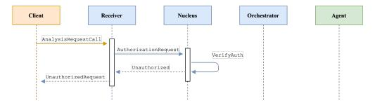
Figure 4.5: Message sequence chart - authorization checking failure
