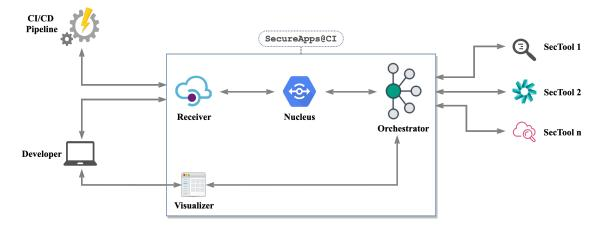
Figure 4.4: Architecture of SecureApps@CI and its integration with CI/CD pipelines, developers and arbitrary, external security analysis tools
