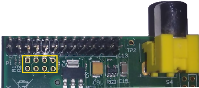
Figure 4.3: GPIO pins of the Raspberry Pi B .
