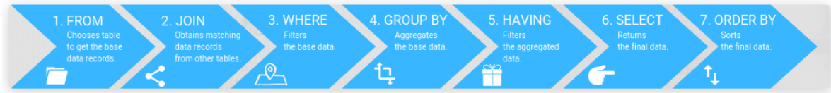
Figure 4.10: Order of execution of each clause in a SQL query [4] on MYSQL, and also used in Presto. May vary depending on the relational DBMS.
