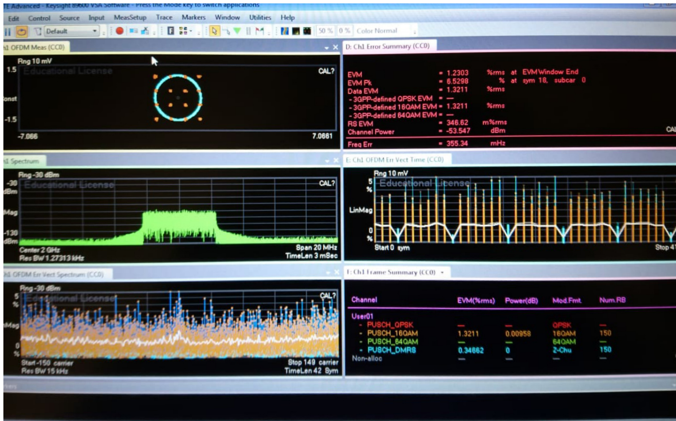
Figure 4.3: VSA with received uplink signal, produced by the Waveform Generator from MATLAB Toolbox.
