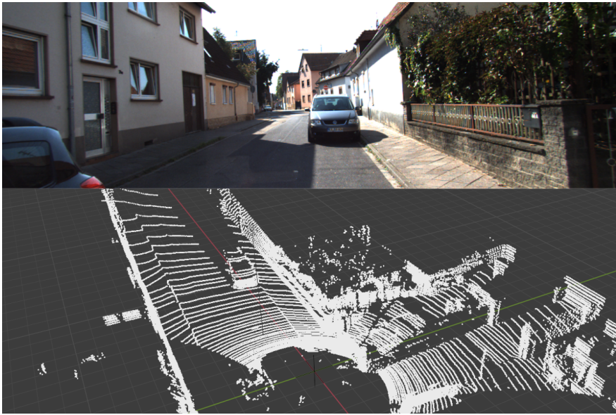
Figure 2.4: Front view and point cloud of a KITTI object detection sample.
