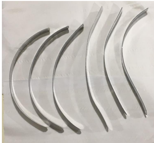
Figure 60: Bending of samples due to ASR with 50% reduction rate, 1 pass (left) and 2 passes (right).
