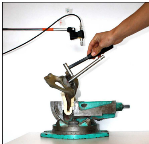
Figure 3.8: Example of in vitro testing of the T1-L3 technology for uncemented fixations of the acoustic approach. The following components are included; artificial pelvis, microphone (suspended above the artificial pelvis), the metal rod (connected to the acetabular cup), and the hammer (used to drive the system). Reprinted from [69] with permission from Elsevier.
