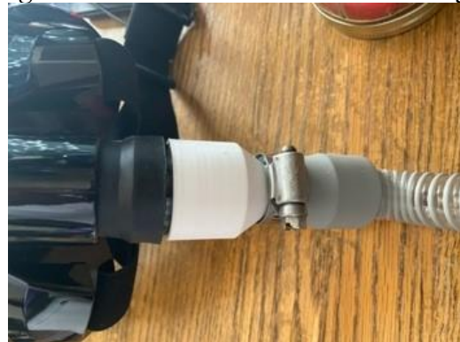
Figure 36. Attachment of snorkel mask to hose.
