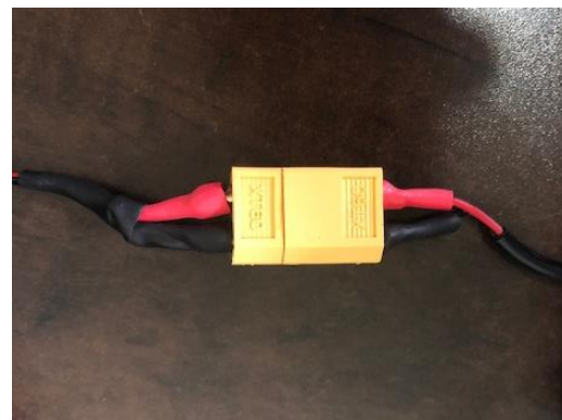
Figure 33. XT60 with wires connected.
