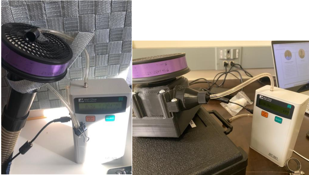
Figure 40. Particle count testing alternative setups.
