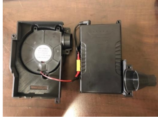
Figure 34. Blower and wiring inside housing.
