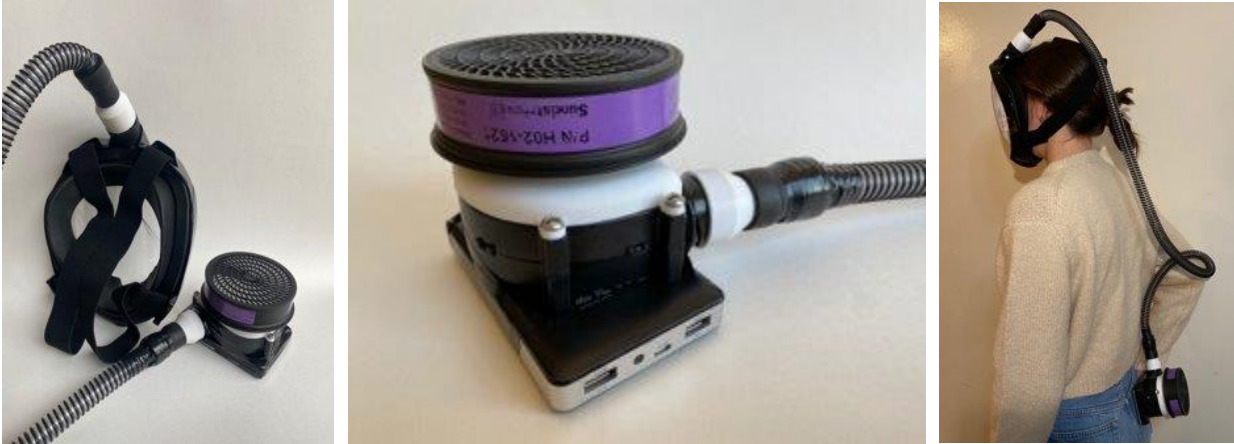
Figure 23. Sealed design structural prototype. From left: the assembly, the battery pack subassembly, and the prototype in use
