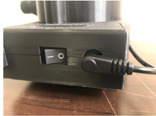
Figure 37. On/Off button with DC cable plugged in.
