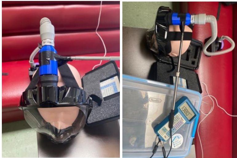
Figure 43. Flowrate verification test.
