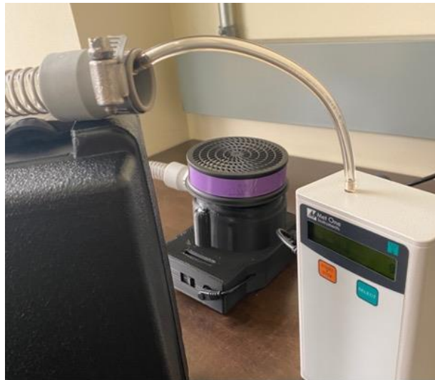
Figure 41. Final particle count test setup.
