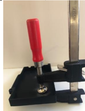
Figure 31. Securing the rivets with a vise.
