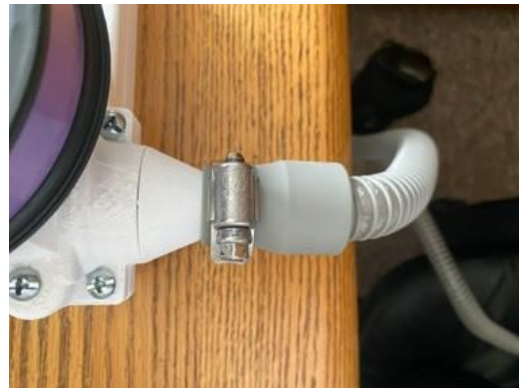
Figure 35. Attachment of hose to housing.
