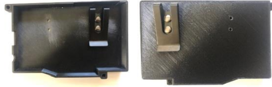
Figure 30. Bottom housing with belt clip and rivets, top on the left, bottom on the right.
