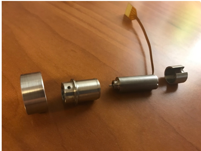
Figure 37. (From left to right) Completed flywheel, motor housing, Maxon motor, and motor endcap
