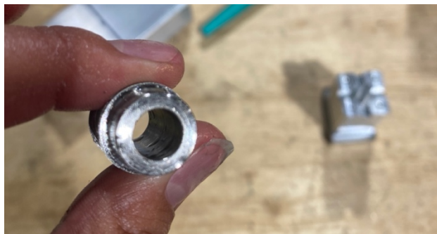
Figure 34. Completed inner bore of motor housing done on manual mill
