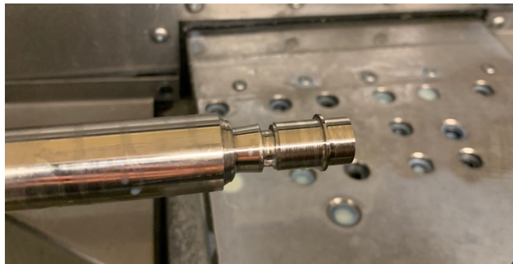
Figure 33. Completed outer operation of inner (motor) housing on CNC
