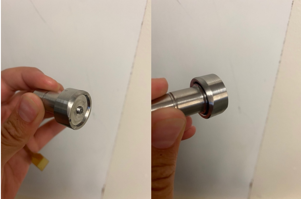
Figure 40. Fly Wheel after Balancing
