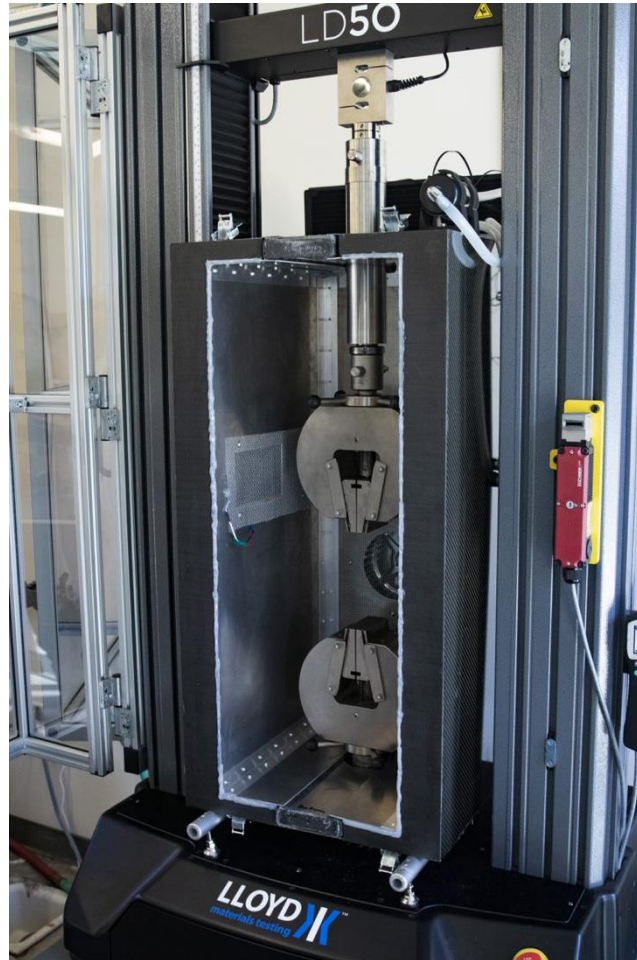
Figure 44: The main chamber with slots installed placed in the LD50.
