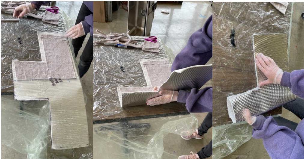
Figure 29: Shows the process of making the insulation pillows from left to right.
