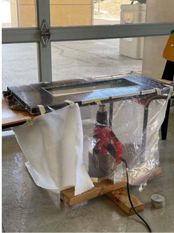
Figure 38: Testing set up for the heat bleed using a heat gun, laser temperature reader, and high temp vacuum bags to prevent convection.
