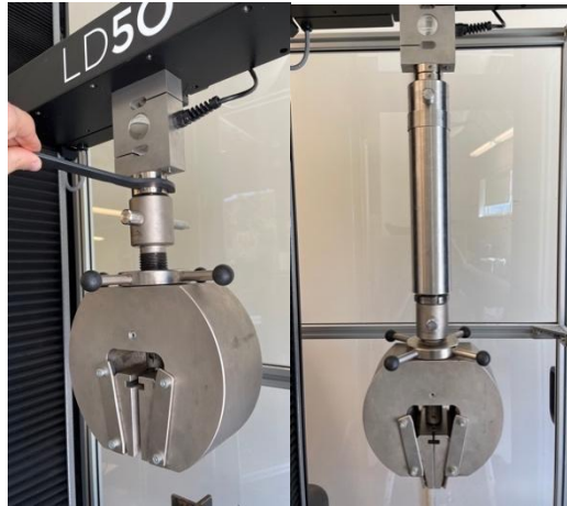
Figure 6: Shows how to add the extender arm to the LD50.
