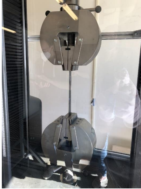
Figure 1: Sample Positioned in clamps with blast shield closed.
