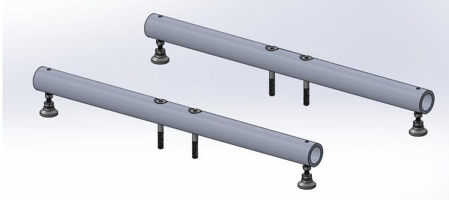
Figure 12. Rail System assembly model.
