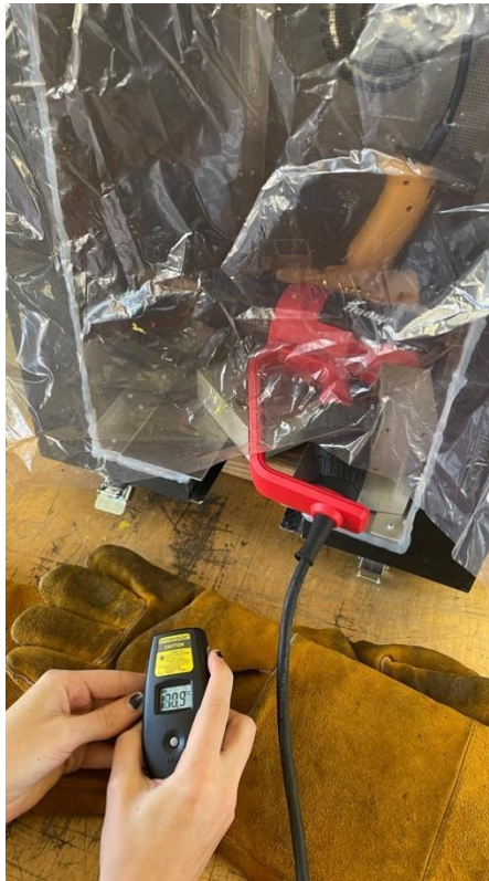
Figure 37: Testing set up for the heat bleed test on the main chamber.
