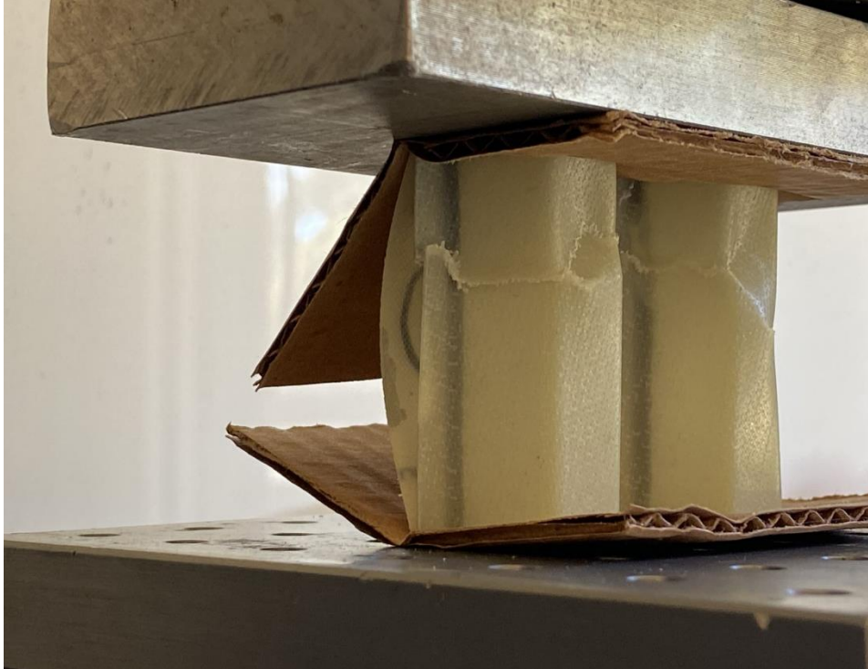
Figure 33: Fiberglass corrugate undergoing compression testing. Failure modes can be seen in the fracturing of the trapezoidal corrugate and separation of the back plate.
