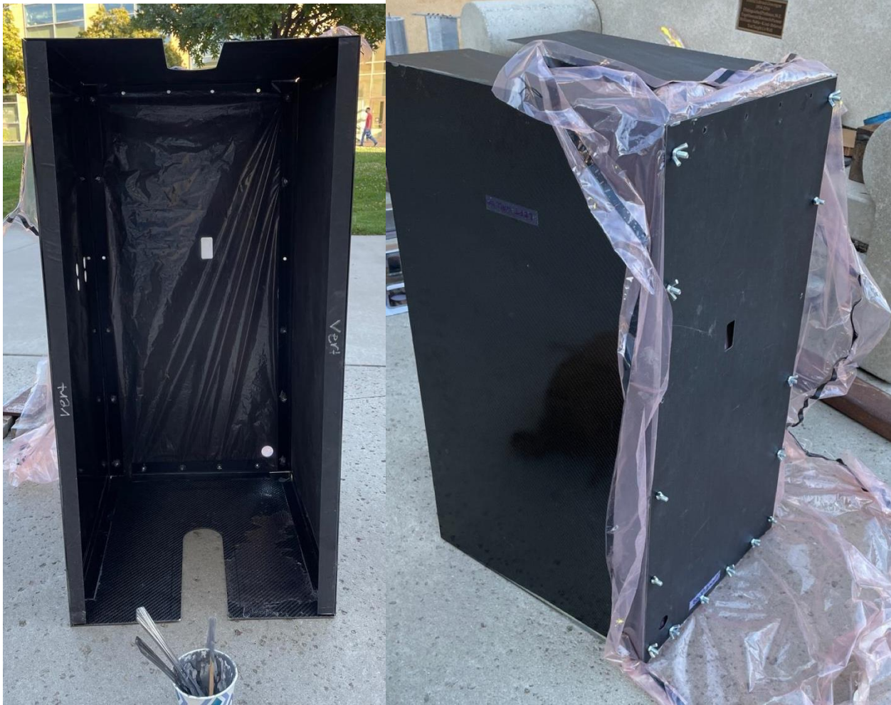
Figure 22: (left) Inner view of the bolt heads being epoxied to the back flanges. (right) Outer view of the vacuum bag being used to prevent the back panel from sealing to the flanges as the wingnuts hold the bolts in place while drying.
