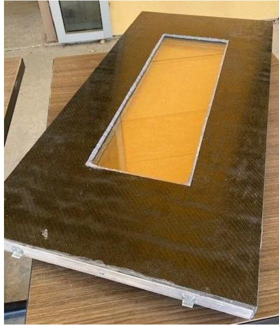
Figure 26: Shows the door after both sides were epoxied together.
