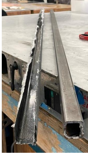
Figure 20: 1 inch u-channel used for structural supports.
