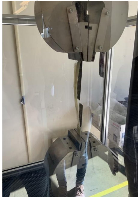
Figure 2: Sample post failure still in clamps and behind safety shield.
