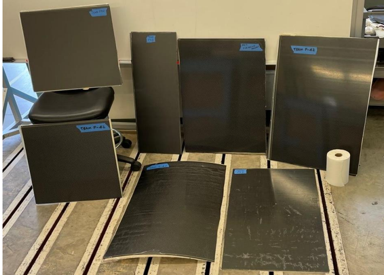
Figure 18: Completed composite panels, pictured before being sent to the waterjet for proper sizing and hole cutting.
