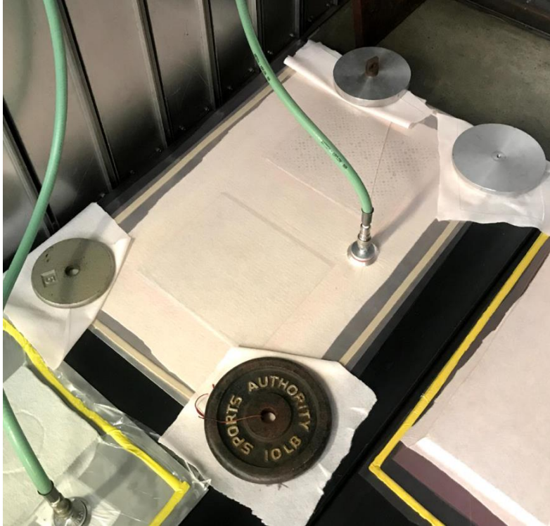
Figure 16: A completed panel layup sealed under a vacuum bag. Weights were placed in the corners to ensure the tacky tape did not lift and let air fill the bag.
