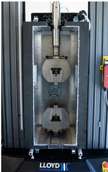
Figure 9: Shows the chamber on the rails and slid into place against the LD50 arms.
