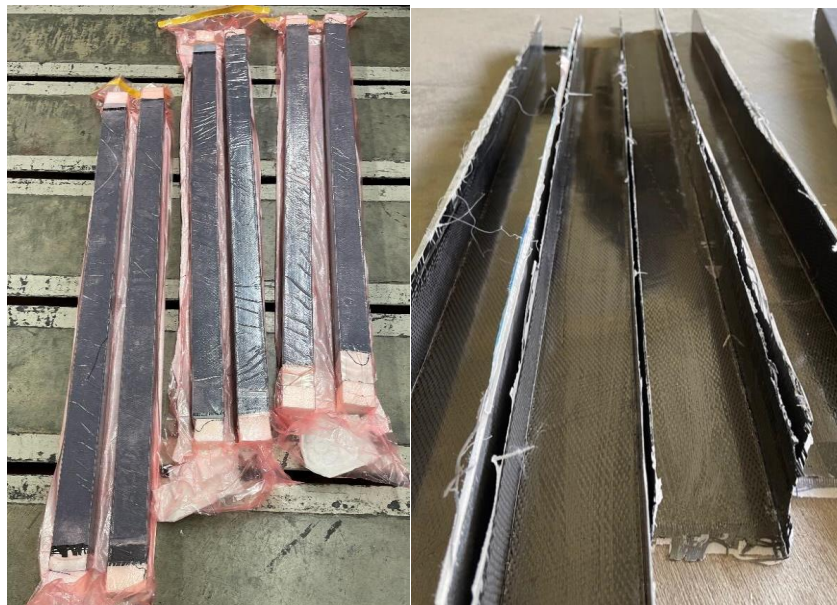
Figure 19: (left) L-brackets vacuum sealed and ready for cure cycle. (right) Brackets out of vacuum bag before cutting into L brackets.
