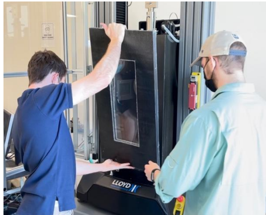
Figure 11: Shows the door being held up into position to attach to the chamber.
