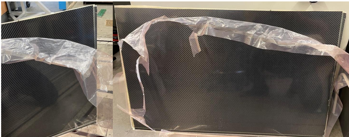
Figure 17: Vacuum bags being peeled off of the shiny surface finish sides of the panels.
