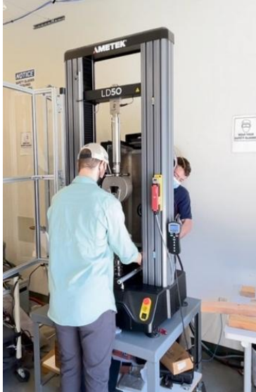
Figure 8: Shows one person lifting the chamber while another ensures it is lined up properly.
