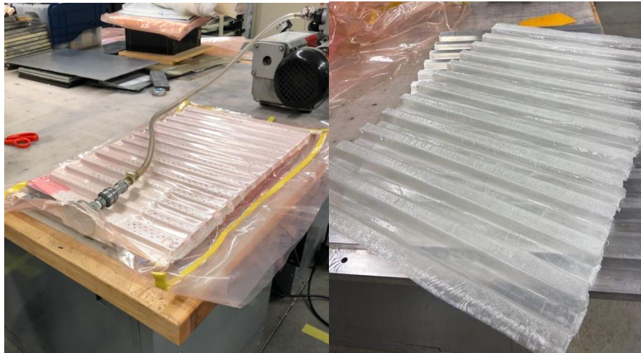
Figure 6. Initial composite wet layup results using a vacuum bag.
