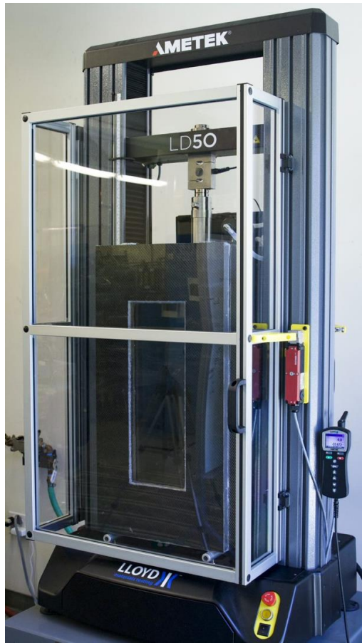
Figure 45: Fully assembled chamber inside the LD50 enclosure.
