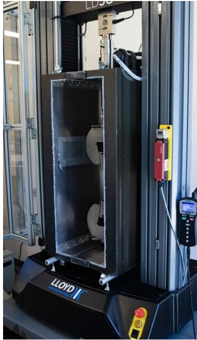
Figure 10: Shows the slots inserted on the top and bottom of the chamber.
