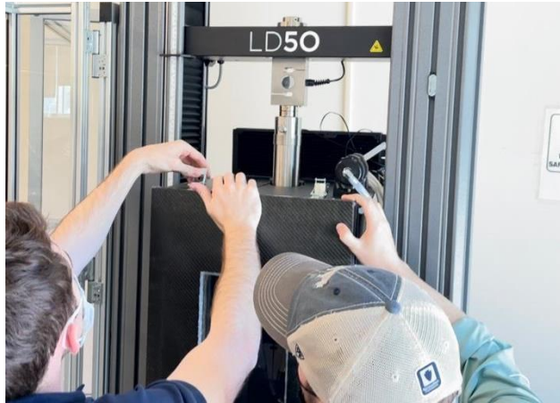
Figure 12: Shows the door latches being fastened to the chamber.
