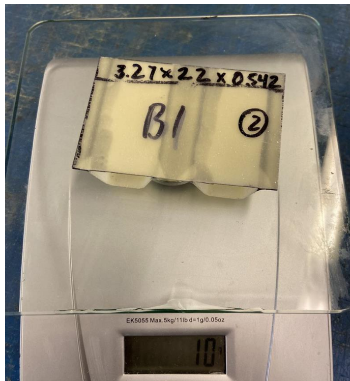
Figure 32: Sample cut piece of fiberglass corrugate to be tested.
