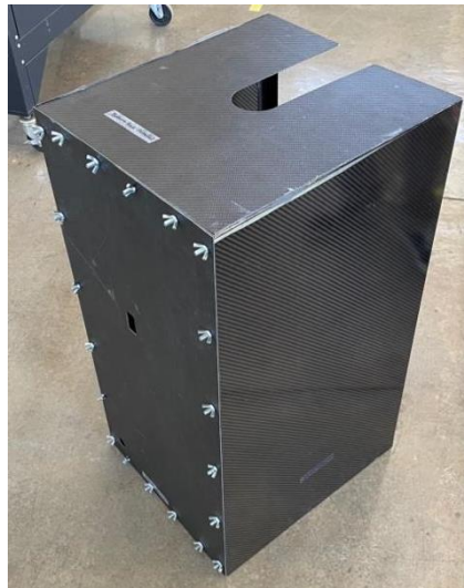
Figure 5: Shows the back panel fully bolted onto the chamber (top 4 middle bolts were later removed and deemed unnecessary along with bolts next to the ducts).
