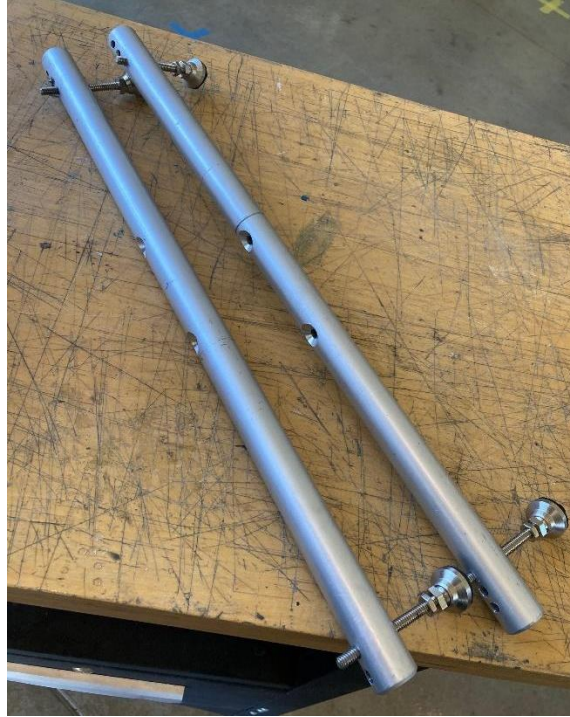
Figure 27: Rails with drilled holes and stool feet installed.
