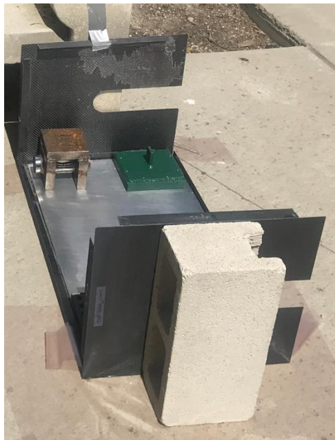
Figure 21: Composite panels being epoxied together using weights and flat surfaces to ensure perpendicularity and good bonding surfaces.
