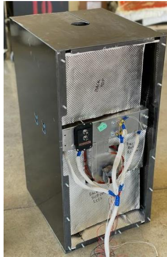
Figure 4: Shows the epoxied bolt locations when the back panel is off.
