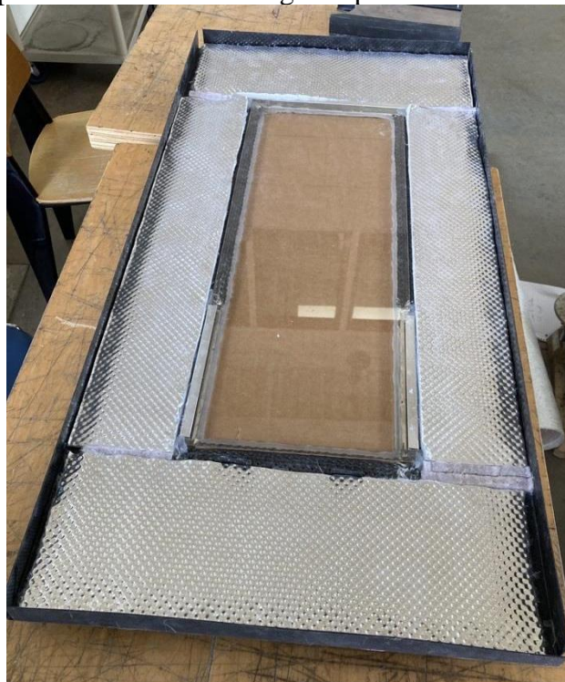
Figure 25: Shows the radiation shield placed around the viewport. Aerogel insulation is below the shiny surface seen.
