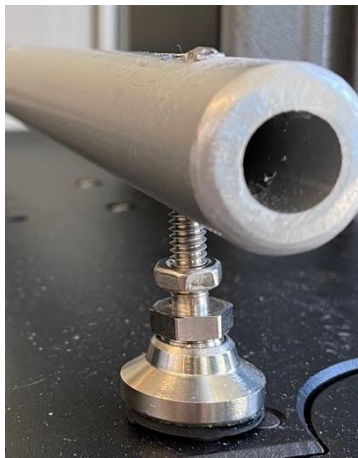
Figure 1: Shows the swivel level mount integration to the rails.
