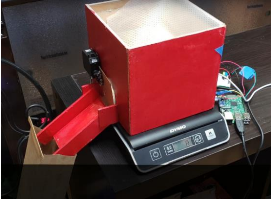
Figure 7. The “Coffee Cube” is an invention created to simplify the bagging process of coffee beans.
