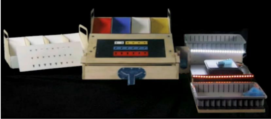
Figure 6. “Sort-a-Screw” is a desktop station that assists with kitting and packaging for different types of screws.
