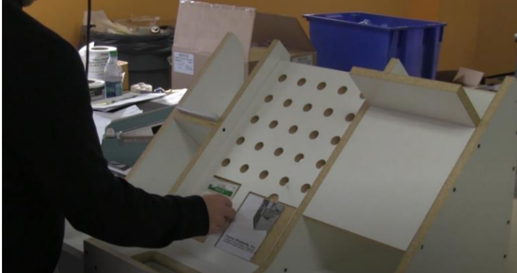
Figure 8. The sorting station was designed for Weaver Industries ProPak to assist in the production and packaging of Fomo nozzles.
