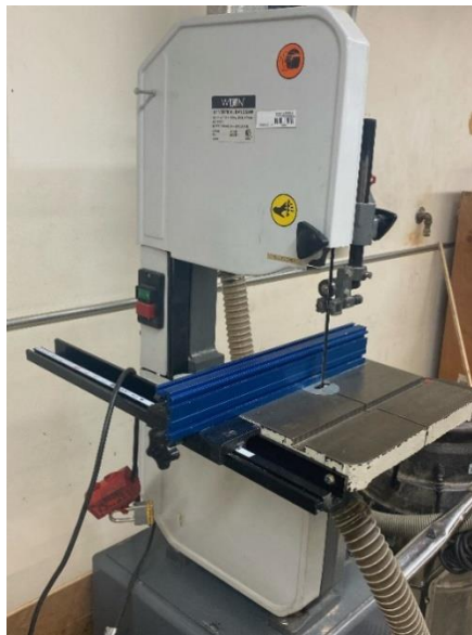
Figure 43. Manufacturing Process – Vertical Bandsaw
