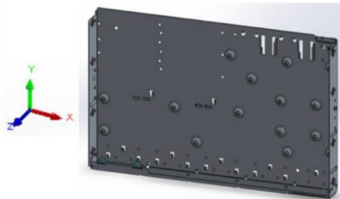
Figure 30. 11.2" Depth Chassis 700-122030-01_02 from Vore CR Non-POE subfamily
