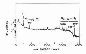
Fig. 3. Deuteron induced  $\gamma\text{-ray}$  spectrum used for measurement of C- and O-losses under bombardment.
