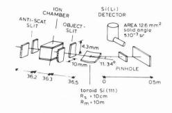
Fig. 7. Schematic layout of the set up used for the development of a synchrotron microprobe
