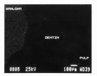
Figure 2. Area map with the window set to illuminate areas with mercury content. The amalgam area is well-defined but the dentin and pulp regions are not. From the same location as Figure 1. Sample was freeze-dried and coated with 20 nm of carbon. limit ( $C_{DL}$ ) for mercury, 9.0 µmg/g. The detection limit was calculated using the Ziebold equation with the Ryder correction (Barbi 1980) as follows:
