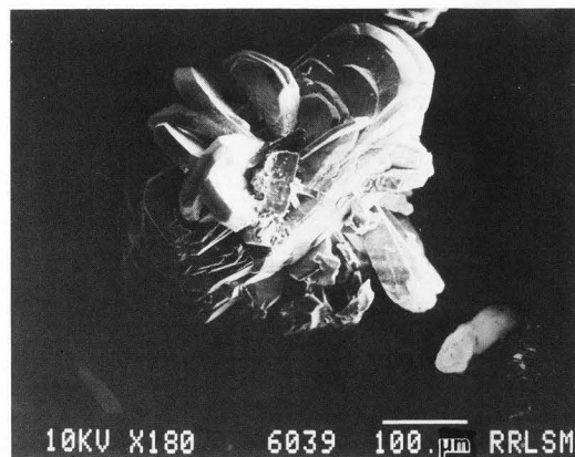
Fig. 2b. Whewellite crystal on addition of citric acid showing distortion of architecture.
