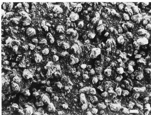
Fig. 3: Surface of polyethylene matrix containing 60% W/W of CaCl 2 . Bar=100 μm.
