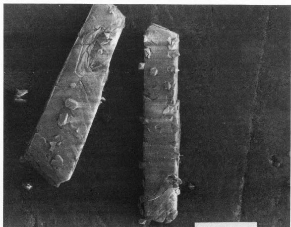
Fig. 13: Transformation from COT to COD at room temperature. Bar=100 \mu\text{m} .
