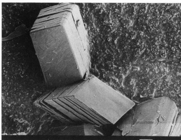
Fig. 12: COT obtained by interfacial crystallization. Bar=10 \mu\text{m} .
