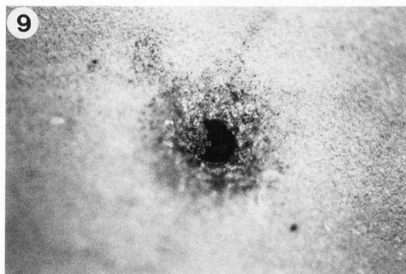
Figure 7: Laser microprobe sampling of a test painting cross section. Crater indicated by arrow at right, approximate diameter is 70 microns. Details of structure in text.
