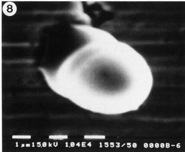
Fig. 8. Aluminum droplet which impacted on copper strip at 71° while still molten.
