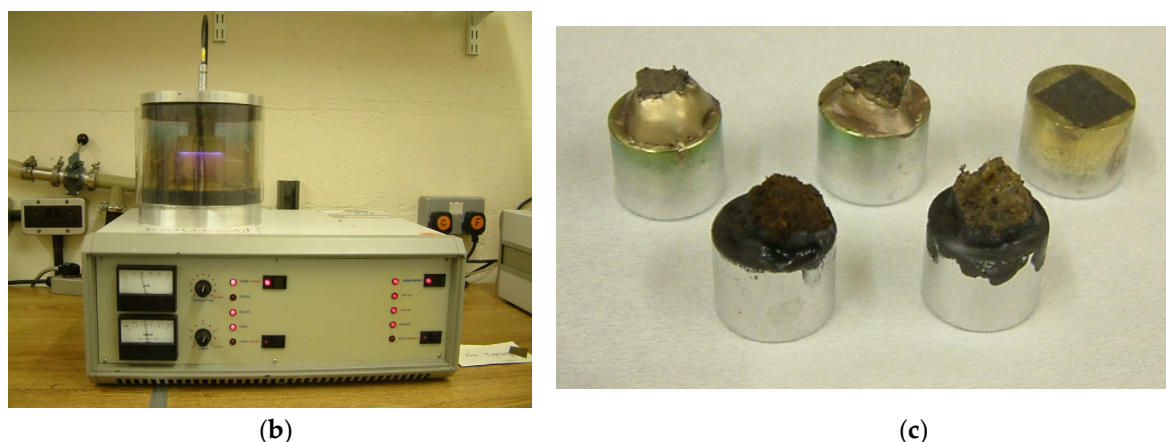
Figure 6. SEM and vacuum coating equipment: (a) SEM's main components, (b) coating of samples with gold and (c) samples before and after coating.
