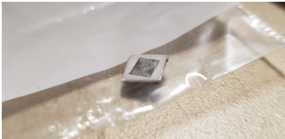
Figure 4.4: Image of the A3 sample with diffusion bonded platinum patch
