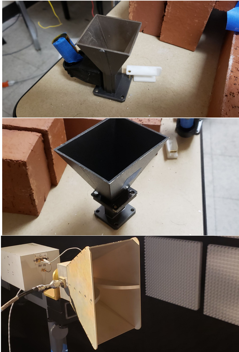
Figure 2.3: (a) 10 dB gain x-band horn antenna. (b) 15 dB gain x-band horn antenna (c) double-ridge wideband horn antenna
