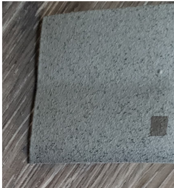
Figure 4.3: Image of PA sample with sintered platinum paste patch before being cut to fit inside the heating pad.
