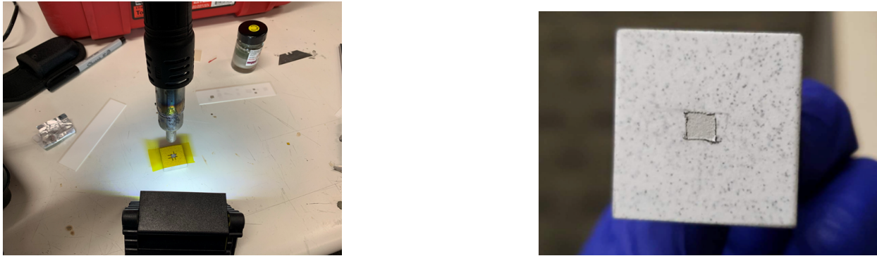
Figure 3.1: (a) the metallization process. (b) the finished A0-4 reflective patch sensor.
