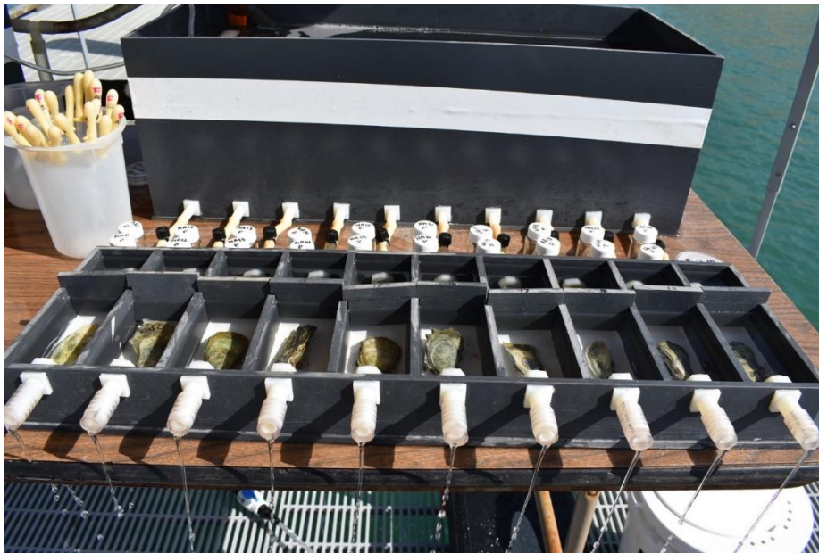
Figure 10. Flow-through filter-feeding bivalve filtration tank used in biodeposition trials.
