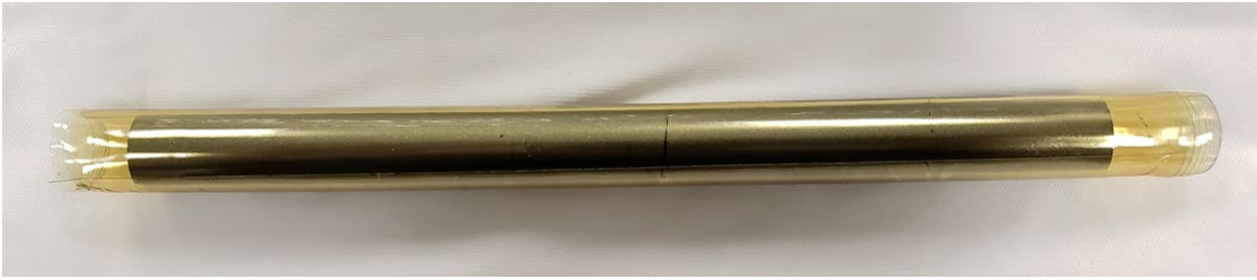
Figure 38: Finished As_{40}Se_{60} fiber preform with pressure crack in the center before being taken to the benchtop fiber draw tower.
