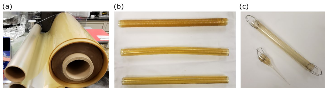
Figure 37: PES (left) and PEI (right) film rolls (a). Consolidated test wraps of PEI at 285°C (top), 280°C (middle), and 275°C (bottom) (b). Pre- and post-draws of consolidated PES tubes for testing tower temperatures (c).
