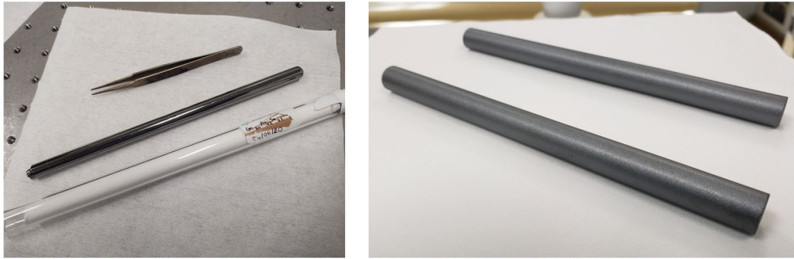
Figure 36: \text{Ge}_{30}\text{As}_{13}\text{Se}_{32}\text{Te}_{25} (left) and \text{As}_{40}\text{Se}_{60} (right) rods, both were 10mm in diameter and 150mm in length. The rod on the left was slightly longer by a few millimeters. Although \text{As}_{40}\text{Se}_{60} rods were unpolished blanks, the glass surface became smooth when drawing.
