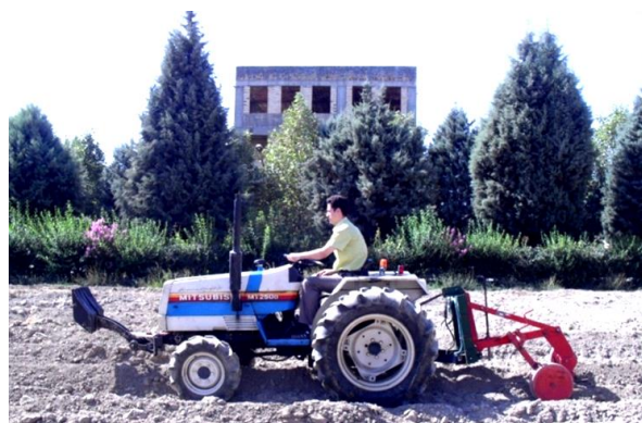
Figure 8. The field testing of Automatic Weight Transfer Control System
