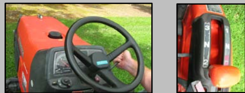
Fig. 3. Left photo: Moving the throttle lever on a tractor by hand to increase or decrease engine speed (RPM) on the tachometer. Right photo: Multiple gear and high/low options are typical of most tractors.
