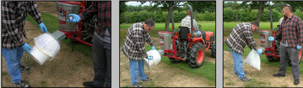
Fig. 8. Left photo: Capturing bait from a Herd® GT-77 spreader using a bucket with a slotted lid with an assistant timing the collection. Middle photo: The bucket collecting method also allows a single person to both collect and time the collection using their leg to keep the bucket in place. Right photo: Holding a collection bag directly on the chute attachment without a bucket. Note that two hands are required to hold the bag in place and that a second person is needed to time with this method.
