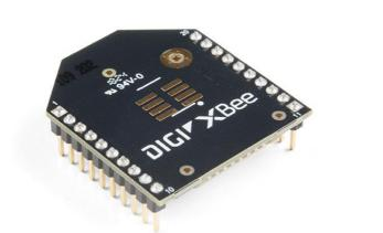
XBEE Module: Responsible for transmitting and receiving sensors data wirelessly between main controller and remote sensor unit. The communication is completely wireless, allowing us to build a waterproof system.
