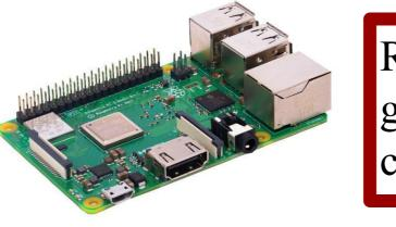
Raspberry Pi: Responsible for calculating moisture and temperature value and running graphic user interface. The raspberry pi are used for both wireless sensor module and coordinator with touchscreens.
